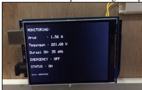
Figure 6. LCD display for current and voltage monitoring
