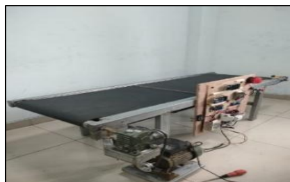
Figure 1. Mock Up Conveyor
