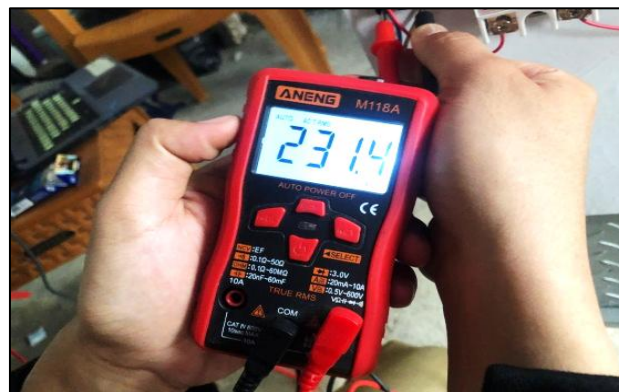
Figure 18. PLN Voltage Testing Source: Author's Documentation
