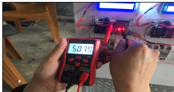
Figure 20. LCD Input Testing
